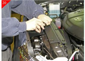
Place shell back on vehicle. Snap the bottom portion of the grille shell in place followed by the (2) 10mm bolts and (2) plastic rivets. Ref steps 1-3
