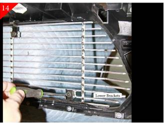
Repeat process for bottom or lower brackets. With holes marked for drilling remove billet grille from opening.
