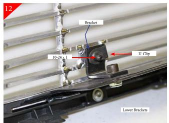
Now attach lower brackets to billet grille again using supplied u-clips and 10-24 x 1 bolts. With brackets attached to grille, place billet grille into opening and center.
