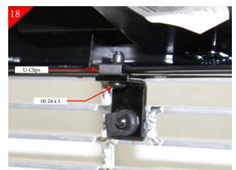
Place <u>billet grille</u> into opening and attach the upper brackets using the supplied 10-24 x 1 bolts as shown.
