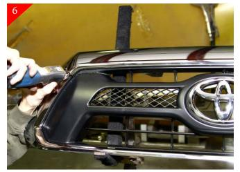
Using the black plastic where it meets the chrome portion of the shell as a guide cut with air saw without cutting into the chrome. Making sure to leave enough material for finish standing.
