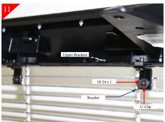
Attached supplied upper brackets to billet grille as shown using u-clips and 10-24 x 1 bolts.
