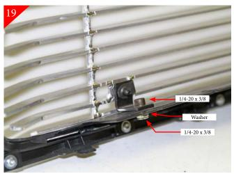
Now attach the lower brackets using the supplied  $1/4-20 \ge 3/4$  bolts and 1/4-20 nyloc nut and washer as shown.
