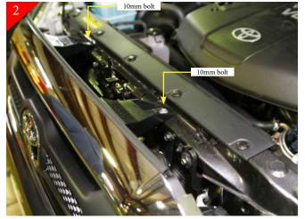
Next remove the (2) 10mm bolts that connects stock shell to core support shown above.
