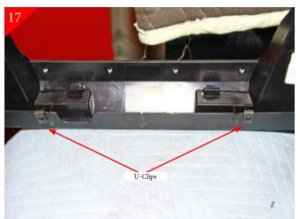
Place supplied U-clips on the just drilled upper bracket attachment points as shown above.
