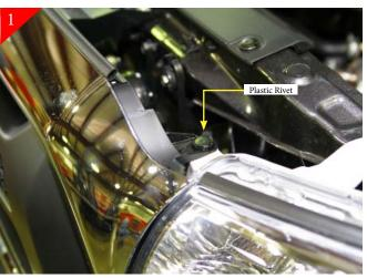
Start by opening and removing the (2) plastic push pull style rivets. Do so by pulling or lifting the center portion of the rivet to release. 1 located on drivers side other on passenger side.
