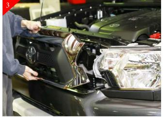
With top portion of shell free. Locate clips along bottom of stock shell and release. Do so by lifting up on the tabs to release. Stock grille shell will be free at this point.
