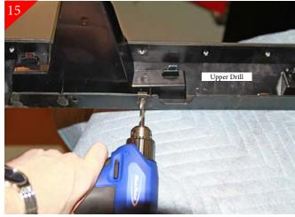
Now using a 1/4" drill bit, drill the just marked locations. You may remove the grille during drilling. Repeat process for all (4) mounting brackets.
