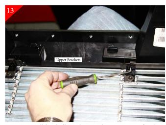
Next you will be drilling the attachment points for the just placed brackets. If necessary use a pair of vice grips to clamp bracket in place while marking holes. Check alignment across the face of the grille make any adjustments. Then using a scribe mark hole locations.
