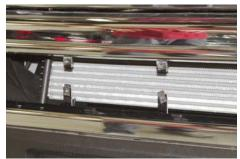
3. Next attach brackets into bumper opening using the stock bolts and stock locations to secure brackets in place. The bend in the brackets go to the inside toward Trans and Intercooler. See (Fig C).
