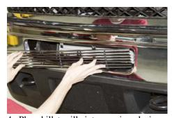
4. Place billet grille into opening placing one in first and pushing past the opening and then bring the opposite end in and slide back. Align mounting tabs in billet grille with the brackets and secure with the supplied 10-24 x 1" bolts. Tighten bolts without over tightening. Note: A drop of red/blue loctite on the bolt threads will significantly reduce the chance of bolts backing out due to road vibrations.
