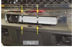
1. Start by locating the (4) stock bolts located in the bumper opening, that you will use for installing the supplied brackets see (Fig A). The yellow arrows are pointing to the stock bolt locations. For the bottom (2) bolts you will need to remove (2) plastic rivets holding rubber weather material that is covering the stock bolts. Using a 7mm ratchet remove the (4) bolts.
