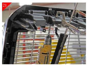
Slightly loosen all the upper brackets so that they will rotate out of the way for drilling. Using a 1/4" drill bit, drill the just marked upper hole locations.
