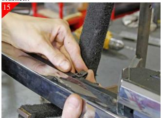
Place supplied u-clips on the just drilled hole locations as shown.
