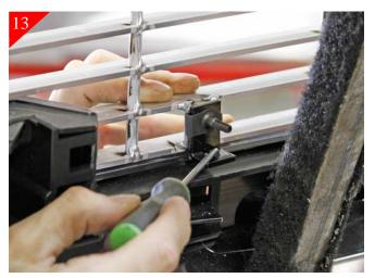
Place billet grille into opening and center. Align the bottom brackets with the backside edge of grille shell and using a scribe mark the hole locations to be drilled. Repeat for all bottom brackets.
