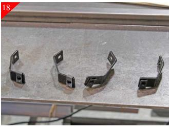
Locate the (4) upper brackets and place the supplied u-clips on the long end of each bracket as shown above. The Larger 2 brackets attach to the center most mounting tabs and the 2 smaller bracket go to the outside mounting tabs.
