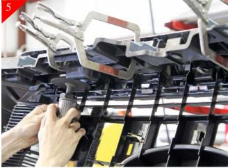
Next you will be removing the center portion of the stock grille shell. Using a cut-off wheel along the top and bottom of the shell cut the vertical attachment points as shown above. (Showing the top)
