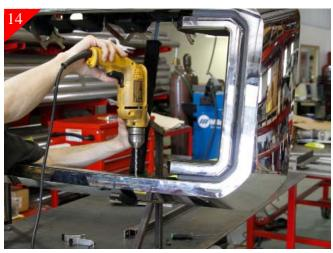
Using a 1/4" drill bit, drill the just marked bottom hole locations.
