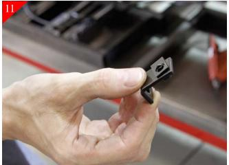
Locate the (4) small brackets and place supplied u-clips on the long end of bracket as shown.
