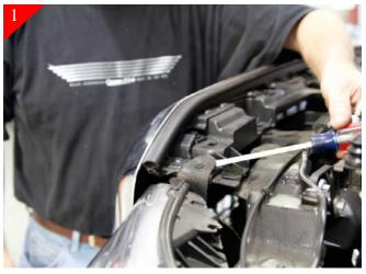
First you will be removing the stock grille shell from vehicle. Do so by removing the bolts across the top of the core support and plastic rivets shown above. The top portion of the shell will be free at this point.
