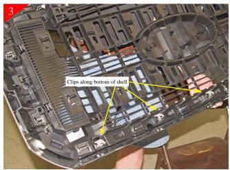
Showing clips along bottom of grille shell after removal.
