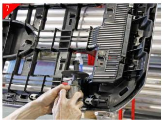
Continue cutting around from the bottom to the side of the grille shell.
