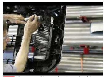
Now you will removing along the sides of the grille shell. Continued from step 7. Repeat for opposite side of shell. Video clip of removing along the side of shell. Double click the picture above to start playback.
