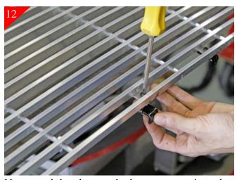
Next attach brackets to the bottom mounting tabs in <u>billet grille</u> using the supplied 10-24 x 1" bolts as shown.
