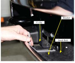
1. Locate the (2) outer most (left & right) stock bolts located in bumper opening and remove. Now locate the (2) supplied "L" shaped lower brackets and place the supplied 10-24 u-clips on the short end of the brackets as shown above. Attach lower brackets in place using the stock bolts that where just removed as shown above.
