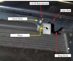
2. Locate the (2) supplied upper brackets and place supplied u-clips on the short ends of the both brackets. Now you will be attaching the brackets. The bolt holes to be used are to the inside of the drop down in sheet metal and larger hole as shown above. Attach using the supplied (2) 1/4-20 x 3/4" bolts and 1/4 nyloc nuts.
