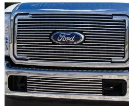
3. With all brackets attached, place billet grille into opening and center. Attach billet grille to the already placed u-clips using the supplied 10-24 x 1 1/2".
