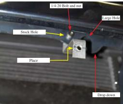
2. Locate the (2) supplied upper brackets and place supplied u-clips on the short ends of the both brackets. Now you will be attaching the brackets. The bolt holes to be used are to the inside of the drop down in sheet metal and larger hole as shown above. Attach using the supplied (2) 1/4-20 x 3/4" bolts and 1/4 nyloc nuts.
