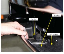
1. Locate the (2) outer most (left & right) stock bolts located in bumper opening and remove. Now locate the (2) supplied "L" shaped lower brackets and place the supplied 10-24 u-clips on the short end of the brackets as shown above. Attach lower brackets in place using the stock bolts that where just removed as shown above.
