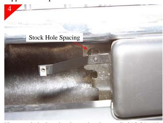
Now attach the long brackets using the supplied 10-24 x 1" bolts. Shown above is the drivers side bracket. Take note as to where the location of the bracket is in the stock hole opening. You will want to have the same amount of open space in the hole for both side of the truck. So push down and to the outside before tightening.
