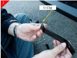
Next locate the (2) long left and right brackets shown above. Then place the supplied U-clips on the short end of both brackets again shown above. Next locate the (2) flat backing tabs and place supplied U-clips on both brackets.
