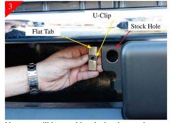
Now you will be attaching the brackets to the truck. Place the flat backing tab behind the stock hole location shown above.
