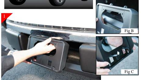
If your vehicle is equipped with a front license frame holder you will need to remove for the install. Do so by releasing the tabs in license frame holder. There are (2) (Fig B) snap clips on the top of the holder and (2) (Fig C) clips in the bottom.
