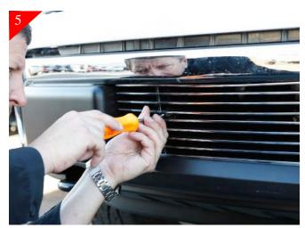
Now test fit the <u>billet grille</u> into the opening. You will need to adjust the long brackets as necessary in order for them to align with the mounting tabs in the billet grille. After necessary adjustments attach billet grille using the supplied 10-24 x 5/8" bolts. Tighten all hardware.
