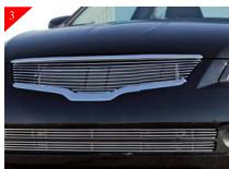
Locate and place the Top billet grille into bumper open-ings and center. Rotate the brackets as necessary to insert the billet grille. The Top billet grille is slightly longer than the bottom also the top grille has an angled bottom bar, this bar goes to the bottom of the top opening. Rotate brackets around so that they catch the plastic in stock bumper opening and tighten. Repeat process for the bottom billet grille.
