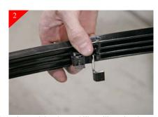
Loosely attach brackets to billet grilles using the supplied #8  $\times$  5/8" Phillips head screws and screwing to the U-clip on brackets as shown above.
