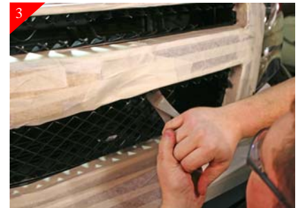
3 Repeat the cutting process for the bottom portion of the stock grille shell as shown above.
