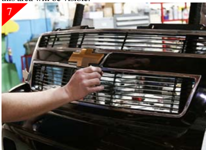
7 Using a scribe or sharpie mark all of the mounting hole locations as shown. Remove billet grille from opening.
