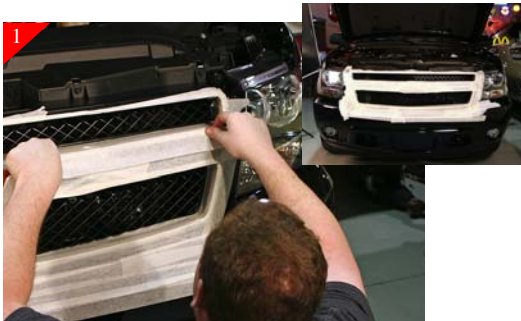
1 Open Hood. Then tape the stock grille shell to protect during install as shown above.
