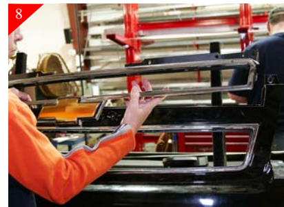
8 Next you will be removing the top portion of the stock grille shell. Do so by removing bolts across top of stock shell. Then reaching behind the stock grille shell, feel along the bottom of the top portion of stock shell for the clips to release see (step 9) for locations and close up of clips.
