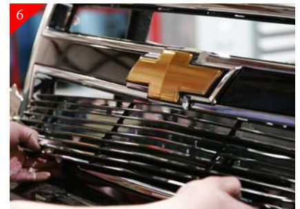
6 Place both the upper and lower billet grilles into opening and center make sure the billet grille is flush against the plastic lip. The bottom portion of billet grille needs to go under the emblem as shown.
