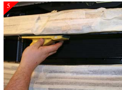
5 After trimming sand all cut areas smooth using a sanding block.
