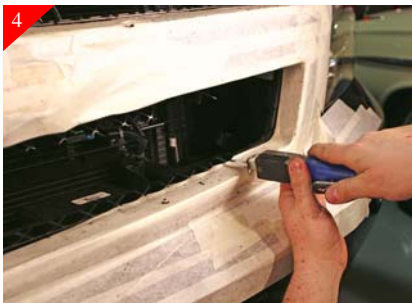
4 Using a hack saw go back and trim all the cut areas or if using a air saw as shown above, take care in trimming as the saw can jump out and scratch painted or chrome surface. Also take care when trimming around the emblem on top portion of stock shell as this area will be visible.
