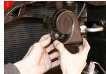
Remove both horns by unclipping the wiring harness and then remove the stock bolt holding in place. This will allow you more room to work.
