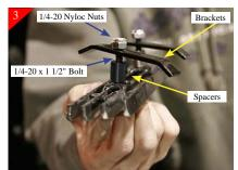
Start by placing supplied  $1/4-20 \ge 1 1/2$ " bolt thru mounting tab in <u>billet grille</u>. Then place the supplied spacers on bolts, followed by the brackets & 1/4-20 nyloc nuts. Repeat process for all remaining billet grilles.
