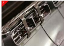
Tighten bolts using an allen wrench and ratchet to
