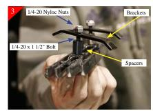
Start by placing supplied 1/4- $20 \times 1 \ 1/2$ " bolt thru mounting tab in <u>billet grille</u>. Then place the supplied spacers on bolts, followed by the brackets & 1/4-20 nyloc nuts. Repeat process for all remaining billet grilles.
