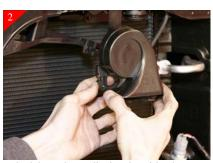
Remove both horns by unclipping the wiring harness and then remove the stock bolt holding in place. This will allow you more room to work.
