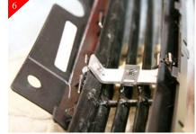
Place supplied u-clips on middle hole of the supplied brackets. Place billet grille into opening and center. Attach brackets to billet grille using the supplied #8 x 5/8" Phillips head screws. Check fitment and mark the hole loactions of the brackets where it meets the stock shell. Remove billet grille from opeing, then using a 3/16" drill bit, drill the just marked locations. Shown above is with the bracket completely attached.
