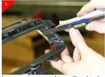
With center poriton removed, you will need to clean up all the cut areas. Using a sanding block to smooth in cleaning up these areas.
