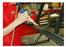
Using a air saw or cut off wheel, remove the center portion of the black plastic backing, leaving some material so that you can do finish sanding, see step 5 for further explanation. out, but you might find it easier to use a utility knife
