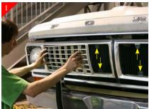
Remove the stock "egg crate" sections by removing the (4) per side screws as shown above. If you are using your old stock shell you will need to remove the inner plastic screw retainers.
