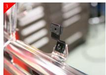
Locate the (2) brackets that have a slightly longer end than the other. These brackets attach to the outer most mounting tab per side in the stock shell. Attach the shorter end to the stock shell using the supplied #8 x 5/8" Phil pan head screws as shown above.
