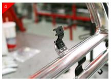
Attach the remaining (2) brackets to the inner (2) mounting tabs in stock shell per side using the supplied #8 x 5/8" Phil pan head screws as shown above.
