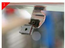
Remove brackets from hardware pack. Place supplied U-clips on all ends of the supplied brackets. Attach the (4) identical Top brackets to mounting tabs in shell using the supplied #8 x 5/8" Phil pan head screws as shown above.
