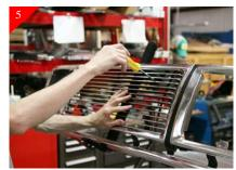
With All brackets attached simply attach billet grille to brackets using the supplied #8 x 5/8" Phil pan head screws.
