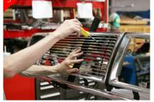
With All brackets attached simply attach <u>billet grille</u> to brackets using the supplied #8 x 5/8" Phil pan head screws.
