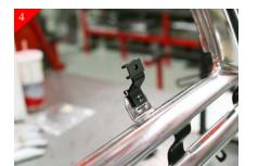
Attach the remaining (2) brackets to the inner (2) mounting tabs in stock shell per side using the supplied #8 x 5/8" Phil pan head screws as shown above.
