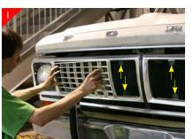
Remove the stock "egg crate" sections by removing the (4) per side screws as shown above. If you are using your old stock shell you will need to remove the inner plastic screw retainers.
