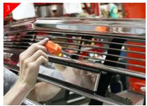
Place top portion of billet grille into opening and align. NOTE: The difference in the (2) billet grilles is that the TOP bar in the bottom portion of billet grille is angled. Attach billet grille to the already placed brackets using  $#8 \times 5/8$ " Phil pan head screws. Now go back and tighten up all the brackets.
