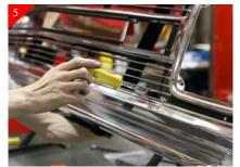
Place bottom portion of <u>billet grille</u> into opening and align. Attach billet grille to the already placed brackets using the supplied #8 x 5/8" Phil pan head screws as shown above.
