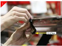
Lay stock shell face down on a protective work surface. Locate the (4) mounting tabs across top of shell and attach Top brackets as shown using 1/4-20 x 3/4" bolts and 1/4-20 nyloc nuts. Do not fully tighten at this point as alignment may be required. Attach supplied U-clips to other end of brackets.
