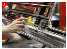
Place bottom portion of <u>billet grille</u> into opening and align. Attach billet grille to the already placed brackets using the supplied #8 x 5/8" Phil pan head screws as shown above.
