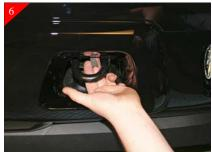
Now attach the brackets to the just marked locations. Attach the top bracket by placing a supplied u-clip on the top side of the tow hook opening as shown above then attach brackets to uclip using #8 x 5/8" Phil pan head screws. Repeat process for the bottom brackets.
