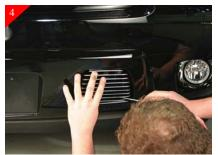
Place billet grille into opening and center. Then using a  $90^{\circ}$  scribe mark the location of the holes in bracket where it meets the vehicle.
