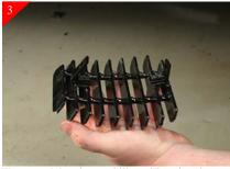
Then attach brackets to billet grille using the supplied  $\#8 \ge 5/8$ " Phil pan head screws as shown above.
