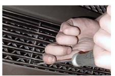
**STEP 4** Next attach the bottom Billet Grille section, by centering the billet grille in opening, and checking that billet grille is properly in place and tighten all supplied toggle bolts.
