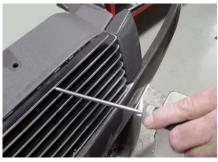
**STEP 3** After Step 2 is completed, move to the top bolts and tighten them, alternating between them to apply pressure evenly. (NOTE: MAKE SURE THE OUTER EDGE OF THE TOP BAR OF THE TOP SECTION IS OVER THE GRAY BEAD AS SHOWN ON THE FACTORY GRILLE.)
