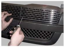
**STEP 2** Check to make sure the grille is properly in place and tighten the lower bolts of the top section of the grille first. It may be necessart to slightly pull down on the center before tightening. (See picture above.)
