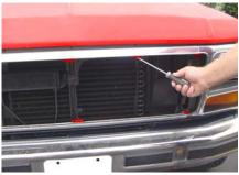
**STEP 1** Remove the stock grille from truck. Using a screw driver remove the 8 screws holding the grille shell to vehicle (shown above in red).
