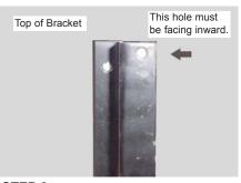
**STEP 2** Next you will be attaching the brackets for mounting the billet grille. Take note of the top hole in bracket this must point inward (Left bracket Shown).
