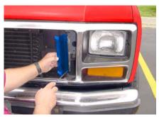
**STEP 3** Attach brackets to vehicle as shown (Bracket shown in Blue). Using factory clips & supplied #8 x 5/8" phillips pan head screws.
