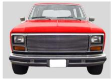
**STEP 5** Attach billet grille to brackets (step 3) using #8 x 5/8" Phillips Pan Head Screws & U-Clips.
