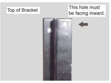
**STEP 2** Next you will be attaching the brackets for mounting the billet grille. Take note of the top hole in bracket this must point inward (Left bracket Shown).
