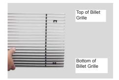
**STEP 4** Next you will be installing the <u>billet grille</u>. Take note that there is a top and bottom to the billet grille. The top (The tab is welded in the 3rd bar). The bottom (The tab is welded in the 2nd bar). Shown
