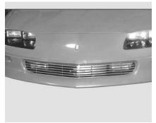
**STEP 3** Attach grill using the supplied  $4 - #10 \times 1 1/4$ " as shown.
