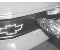
STEP 2 Drill 1/8" hole at each marked location.
