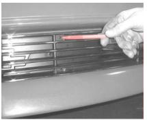
**STEP 1** Place <u>grille</u> into bumper and center. The grille will set inside the I.D. of the opening.
