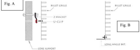
Step 3: Attach the (2) Long Angle Brackets to the 2-center tabs on bottom of <u>billet grille</u> as shown above (Fig. B). Step 4: Attach the (2) Short Angle Brackets to the 2-outer tabs on bottom of billet grille. Attach same as (Fig. B). Step 5: Center Billet Grille in car and mark center line of brackets on car's core support & drill a 9/32" hole in each marked location. Use ¼-20 bolts & nuts to attach.
