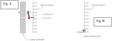
Step 3: Attach the (2) Long Angle Brackets to the 2-center tabs on bottom of <u>billet grille</u> as shown above (Fig. B). Step 4: Attach the (2) Short Angle Brackets to the 2-outer tabs on bottom of billet grille. Attach same as (Fig. B).
