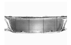
**STEP 6** Now carefully place the <u>billet grille</u> into the back of grille shell. Center the grille in the opening. Mark the eight locations where the 1/4" rods meet the factory shell as shown above.
