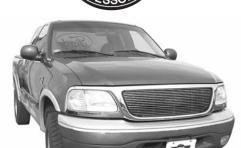
**STEP 1** Remove stock grille shell from vehicle by removing the 6 plastic screws from the core support cover.
