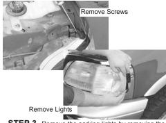
STEP 3 Remove the parking lights by removing the torque screws as shown above. Then lightly pull the parking lights out.
