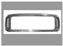
**STEP 3** Cut out the grey plastic center of the grille shell being careful to follow the small grey molded line described in step 2. After cutting the center out use a file to smooth out the edges. Again being careful to follow the grey molded line. NOTE: If installing center only skip step 4. You don't need to cut out the left and right pockets.
