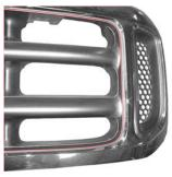
**STEP 2** Place grille on protective work surface such as a work bench with a blanket. Then tape off the chrome portion of the grille with masking tape so you don't scratch the face of the grille shell. Notice that there is a molded line in the shell about 1/8" inside the chrome as shown above.
