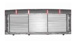
**STEP 4** Attach upper brackets to billet grille using 1/4-20 nuts & bolts. Lay grille shell face down and center billet grille in opening. Mark location of rods as shown above. Drill an 1/8" hole in each marked locations. Now attach grille, buy using self tapping screw in each of the drilled locations. Snap grille shell with billet grille into place. Mark and drill an 1/8" hole in each bracket location. Attach upper with 3/4" self tapping screw, in each drilled location.
