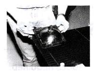
**STEP 7** Slip the parking light under the L-shaped tab attached to the grille.
