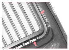
STEP 2 Remove the center section of grille shell by using a cut-off wheel. Cut along the outer most edge of grille shell as shown above.
