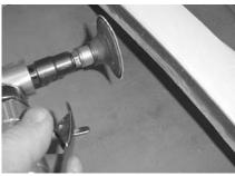
STEP 3 After removing center section grind or sand smooth all rough areas.
