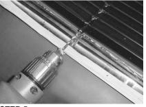
STEP 5 Set Billet grille into grille shell. Then mark center locations of each of the vertical rods of billet grille. Then drill a 1/8" hole at each location.
