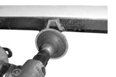
STEP 4 Using a sander or sanding block sand all rough edges smooth. Repaint if neccessary.
