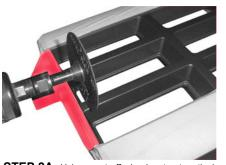
STEP 2A Using a cut-off wheel, cut out vertical and horizontal bars of stock shell.
