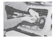
STEP 2 With a cutoff wheel or saber saw, cut out the egg-crate insert from the original grille.
