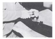
STEP 3 Grind the insert attachment points down smooth.
