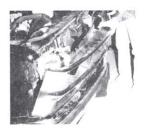
STEP 1 Remove parking lights, remove the grille. There are four 7 mm screws across the top and one screw at the upper center.
