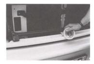
STEP 1 Remove the grille by removing four screws on top and one in the center. Put masking tape on the lower panel in the four mounting tab locations so marks for mounting holes can be seen and to protect the finish when drilling.
