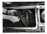
STEP 2 Remove grille support brackets. One located on each side of grille opening. Six 1/2" bolts hold these in place.
