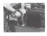
**STEP 5** Remove the grille and drill a 1/4" hole on each side for the mounting brackets.
