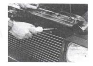
**STEP 9** Install the Phillips screws provided to hold the top grille brackets, and tighten the bolts holding the brackets to the grille.
