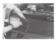
**STEP 4** Position the new grille, centered in the opening and flush with the front surface of the headlight doors. Reach behind and mark through the holes in the mounting tabs.
