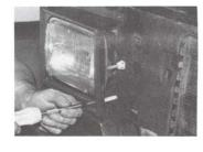
STEP 2 Install long screws provided to hold the headlight doors in position.
