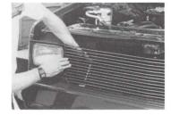
STEP 4 Position the new grille, centered in the opening and flush with the front surface of the headlight doors. Reach behind and mark through the holes in the mounting tabs.
