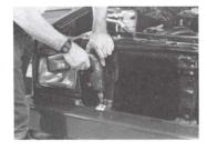
STEP 5 Remove the grille and drill a 1/4" hole on each side for the mounting brackets.
