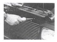
STEP 9 Install the Phillips screws provided to hold the top grille brackets, and tighten the bolts holding the brackets to the grille.
