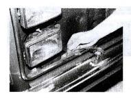
STEP 11 Install clips provided onto lower corners of the grille opening, if needed.
