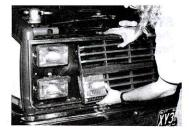
STEP 3 Push the top of the grille in and pull bottom out to remove.
