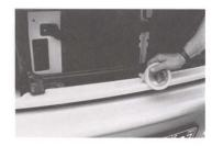
STEP 1 Remove the grille by removing four screws on top and one in the center. Put masking tape on the lower panel in the four mounting tab locations so marks for mounting holes can be seen and to protect the finish when drilling.
