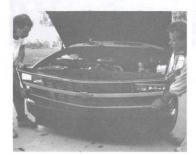
STEP 1 Remove the grille. There are four screws across the top under the hood, one at the bottom center and one behind each parking lens.
