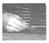
STEP 12 Again trial fit the insert. Be sure the bars are flush with the face of the grille shell in front, and note any place where the frame needs additional trimming. Then mark where the upright bars contact the outer frame.
