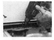
STEP 8 Drill 1/8" holes in the frame at each of these points. When all holes are drilled and the grille checked for fit, the reworked frame should be painted body color or '87-90 GM accent charcoal poly, Code #58.
