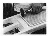
STEP 2 With a die grinder (a saber saw, hack saw or diagonal cutters can also be used), cut out the grille bars just inside the inner rim. Be careful not to cut into the rim.
