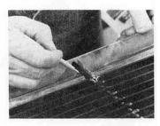
STEP 5 Trial fit the new grille and mark where the round vertical support bars intersect the horizontal bars on the top and bottom of the grille opening.
