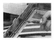
STEP 6 With a rotary tool (or rat-tail file), grind notches into the horizontal bars about 5/8" deep. Check the grille and adjust the depth of the notches so it fits flush with the front of the grille panel.
