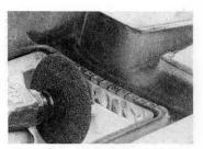
STEP 3 After the bars are removed, grind the remaining nubs on the inside of the rim down even.
