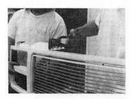
STEP 9 Install the grille by attaching the vertical support bars to the frame with the pop rivets supplied. Reinstall the entire grille unit in the truck.
