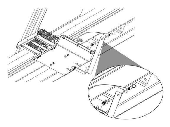
3. Take the entire step assembly and lift it up inside the vehicle behind the side door. It is highly recommended to use a floor jack or something to rest the step assembly on while completing this step. Make sure the Rear Steel Bracket is up against the middle cross member as shown. Take the ½" hardware and assemble it to the vehicle but only hand tighten. This ½" bolt assembly will be tightened in step 7.
