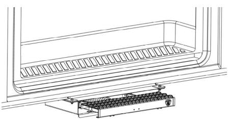
7. Now your step is ready to go. Push the step in to lock in its closed position. Push it again to deploy it. We recommend using a garage door opener silicone spray on the rails from time to time to insure smooth operation of the step.
