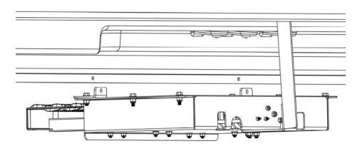
5. Lower the front end of the step down to expose the marked holes. Take a drill motor (a right-angled drill motor will make this easier) with an 11/32" drill bit and drill out the marked holes. Remove all burrs.
