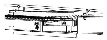
7. Remove the bolt assemblies that hold the "C" shaped steel brackets to the pan. Take the cover plate and slide it between the pan and the "C" shaped steel brackets. Align the holes and reinstall the bolt assemblies just removed. Take the remaining 5/16" X ¾" bolts with washers and nylon lock nuts and securely tighten the cover plate to the pan.
