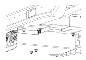
11. Once all the hardware has been installed, securely tighten the step assembly to your vehicle. Push on the step to deploy it. Then push it in to lock it in place.
