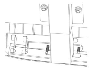
2. From underneath the rear bumper on the passenger side, slide the Long "L" Bracket up above the channel on the vehicle as shown. Insert one of the short carriage bolts on the end of the Long "L" Bracket.
