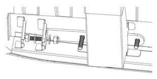
3. Take one of the hex head bolts with two washers and a nylon lock nut and hand-tighten this hardware to the vehicle and the Long "L" Bracket shown in the diagram.
