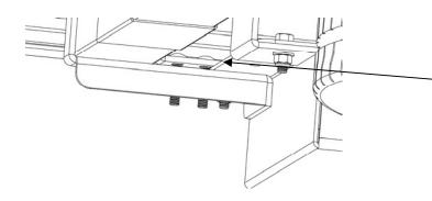
9. Make sure the feet of the "C" Brackets from Step 4, on both sides, are on top of the flange of the black powder coated pan.
