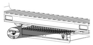
10. Take two 5/16" hex bolts with washers and insert them in the front holes of the Main Brackets so they go through the pan. The first bolt and washer will be fairly easy to install. The second one may be more difficult. Wiggle the entire assembly if the fit is tight until the bolt and washer are installed. Take two washers and two nylon lock nuts and hand-tighten to these bolts.
