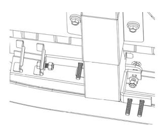
4. Take one of the "C" Brackets and slide it on to the shorter carriage bolt with a washer and nylon lock nut and only hand-tighten. Place two additional longer carriage bolts through the two holes at the bottom of the "C" Bracket. See diagram.
