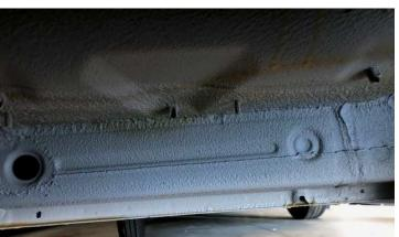
3. With both holes marked, center punch both marks and drill out with the 1/8" drill bit followed by the 5/16" drill bit. Try to clean out burs as best as possible. The step and brackets will need to be disassembled for the next step.
