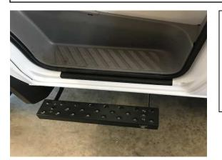
6. Re-install your step and with the 3/16" Allen wrench and ½" socket fully tighten all four button head screws.
