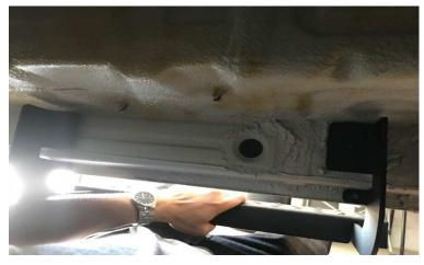
2. With step assembled, place step in the desired location avoiding any bumps or indents to allow both brackets to be parallel to each other. With a marker mark both holes for the 5/16" mounting hardware; top holes do not need to be marked. Excess caulking will have to be cut to allow better fitment of brackets.
