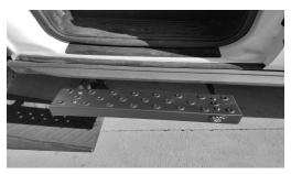
6. Re-install your step and with the 3/16" Allen wrench and ½" socket fully tighten all four button head screws.
