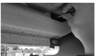
7. Fully tighten both 5/16" bolts to U-nuts. Finally with a 3/8" socket install the #14 self-tapping screws to both brackets and be careful not to over tighten them. Your step is now fully installed follow the same procedure for other side.
