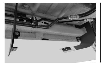
5. With both Unuts in place use the 5/16" bolts and washers to secure both brackets to the rocker panel.
