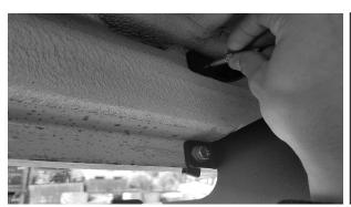
7. Fully tighten both 5/16" bolts to U-nuts. Finally with a 3/8" socket install the #14 self-tapping screws to both brackets and be careful not to over tighten them. Your step is now fully installed.
