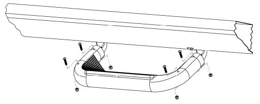
4. Place the Step Casting on the Mounting Brackets. Take the ¼" hardware provided and hand tighten the hardware.
