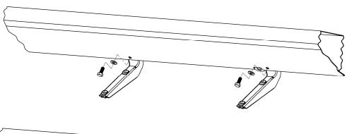
6. Once again, remove the DEF tank cover. Also remove the Step Casting from the Mounting Brackets. Move the Mounting Brackets to the side. Center punch the center of each cross-hair mark. Drill out the centers with a 1/8" drill bit and then go back and drill out the holes with a 11/32" drill bit. Remove all burrs. Refer to Step 8 on Page 2 for installing 5/16" hardware.
