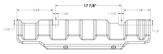
2. With the dimension provided, cut the two slots out on this cover. It is recommended to use a Dremel or similar tool to grind these slots. Cutting with a saw may crack the plastic.
