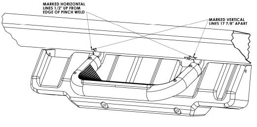
5. Reinstall the DEF tank cover. Slide the Mounting Bracket/Step Casting assembly so that the back of the Mounting Brackets line up with the slots in the DEF tank cover. Mark the lines on the vehicle's body metal as indicated on the drawing. Make sure the 17 7/8" vertical lines are on center with the Mounting Brackets.
