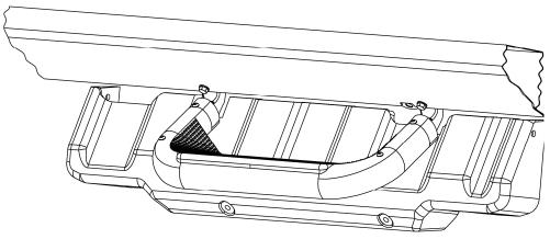
7. Reinstall the DEF tank cover. Refer to Steps 9-13 on Page 2 for final installation of this and all others steps. NOTE: To insure both steps are in a similar position on the front doors, when installing the front driver Super Hoop step refer to the position of the step that you just installed on the front passenger side.
