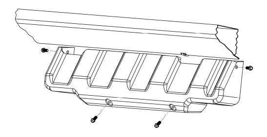
1. Under the passenger front door, remove the black DEF plastic tank cover from your vehicle. You will need a 10mm socket to remove the four bolts. Keep these bolts for reinstallation.
