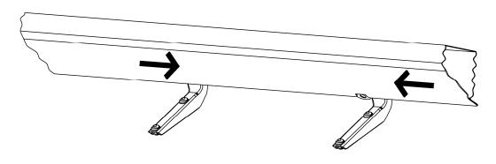
3. Slide the Mounting Brackets behind the rocker panel and in front of the DEF tank as indicated. Move the right Mounting Bracket up against the tab as shown in the diagram. Both Mounting Brackets can be moved forward if desired for a different placement
