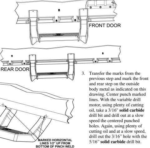
4. Take the 5/16" hardware provided and securely mount the step assembly to the body of the vehicle. Do not use any flat washer under the 5/16" nylon nuts. Using the top ½" holes in each steel mounting bracket as a guide, drill out each hole with a 3/16" drill bit. Install the four sheet metals screws as indicated using the flat blade screwdriver or the 5/16 socket. Now your steps are ready to go! Repeat the same steps for the passenger side.
